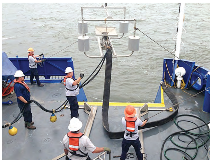
Oil skimmer deployment by an Oil Spill Removal Organization (OSRO) during a drill exercise.
